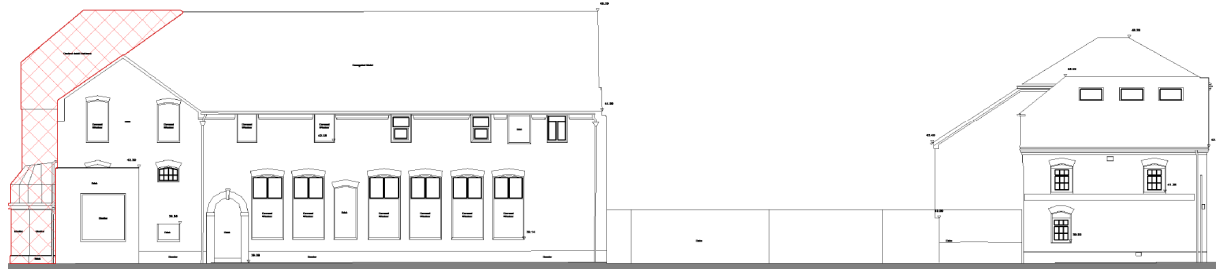
Northfield Road elevation - demolition shown in red
