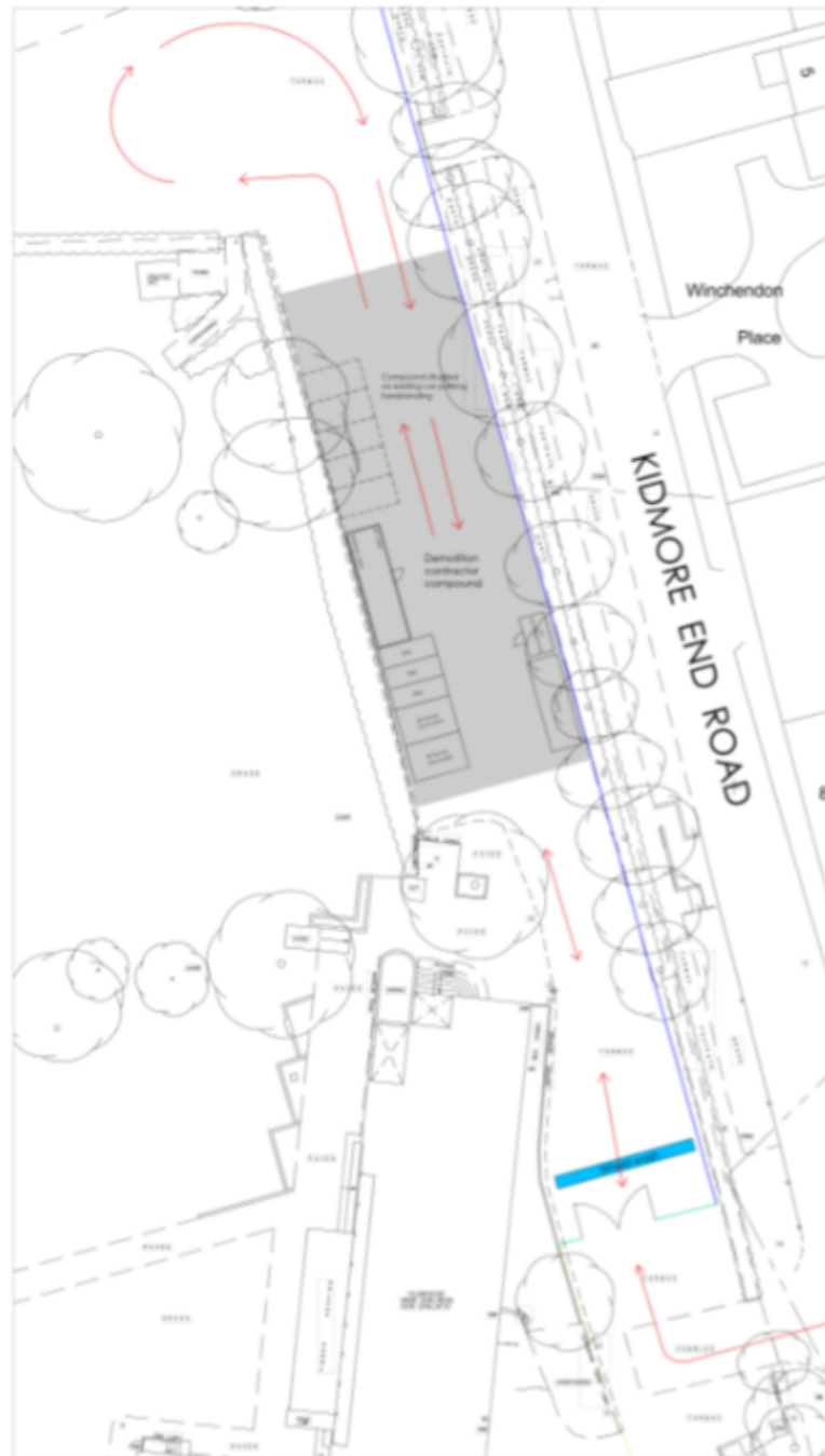
Demolition Plan (Appendix B of the CMS)
